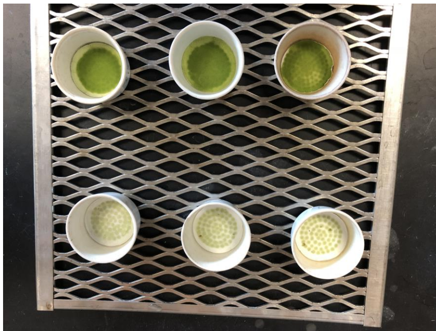
Figure 10. Algal biomass retained on crucible filters for a conventional stormwater pond (top) and a naturalized stormwater pond (bottom) 17 years post-construction 1 .
