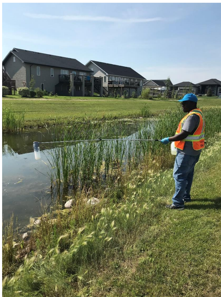
Figure 3. Water sampling from shore with extendable pole.
