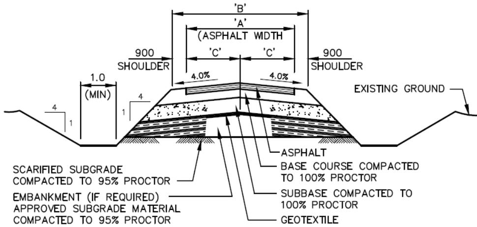
TYPICAL DITCH ROAD CROSS SECTION
